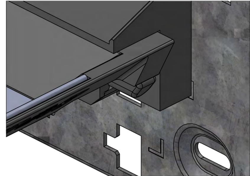
**Step 04:** Support the bottom of the DripShield while moving to the opposite side of the compartment. Repeat steps 01, 02, and 03 on the opposite side of the compartment to complete the DripShield Installation. Gently test that the DripShield is secure.
