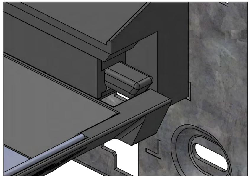
**Step 03:** Push the DripShield from the bottom past the spring loaded latches to secure in place. The latches will move out of the way of the DripShield automatically and snap back to secure the end of the DripShield in place.
