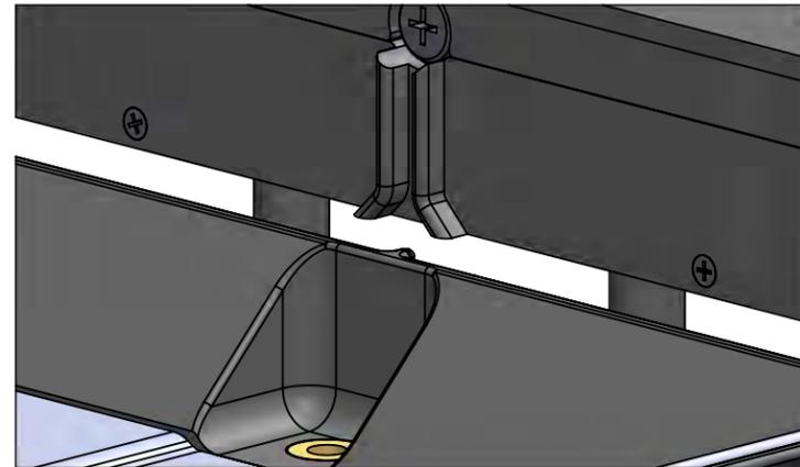
**Step 02:** Slide the DripShield up so that the angled surface on the DripShield end cap is in contact with the latches
