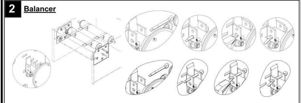
Place the balancer onto the mounting plates. Install cotter pins in holes above shaft on right and through shaft hole on left. Bend cotter pin legs outwards to secure.
