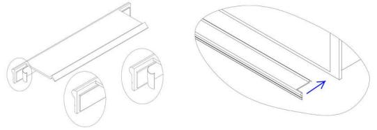
Peel adhesive back and stick sill plate to the compartment's bottom edge.
