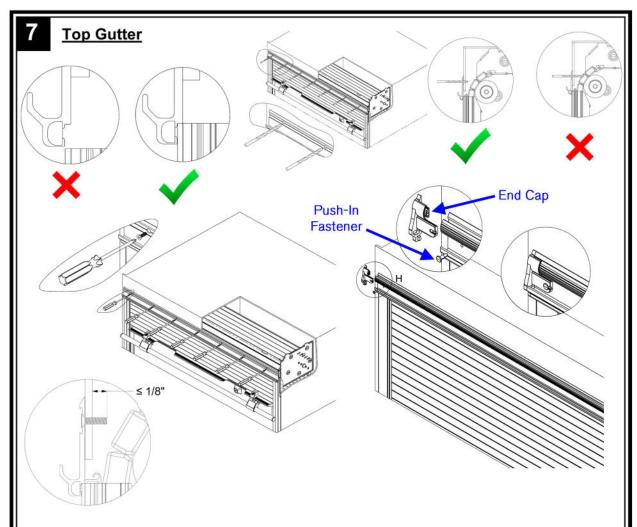
Slide top gutter onto the top edge of both side frames. Drill holes and secure in place with screws. Screws should not protrude more than 1/8" into compartment.
